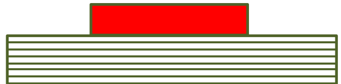
Figure 8. HP disc-shaped specimen with hot surface (in red). Lines represent binder print orientation.
