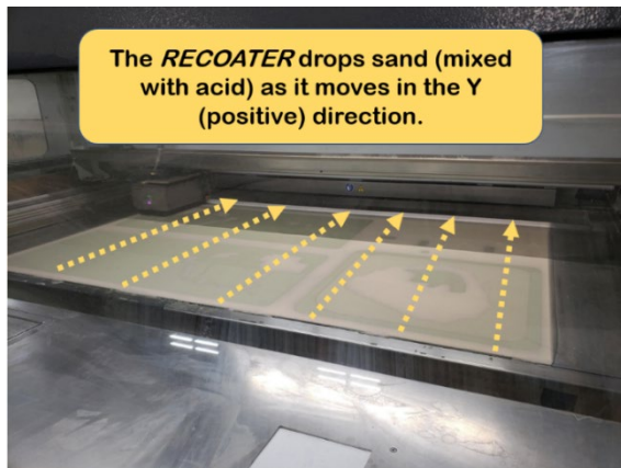
Figure 5. Recoater motion direction is shown with arrows.
