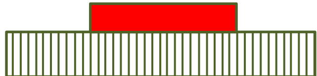
Figure 9. VP disc-shaped specimen with hot surface (in red). Lines represent binder print orientation.
